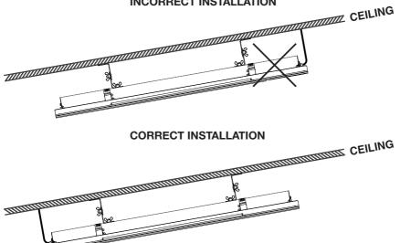
The supply cable must be at the lower end of the heater if the heater is installed at an angle or vertically.
