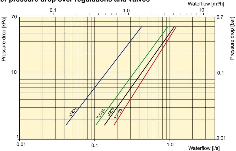
The pressure drop is referring to the mean water temperature 70°C, (PVV 80/60).
